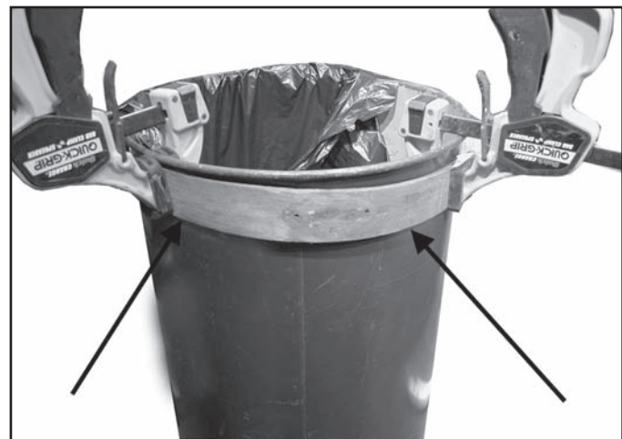
After the oak slat has been steamed in the box we clamp it to a steel drum while it sets.
