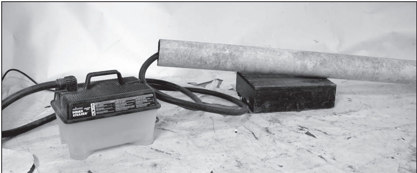
A homemade steam box using a length of PVC pipe and a Warner wallpaper steamer. Seal both ends with rags. Notice the tilt to let the condensed vapors run out.
